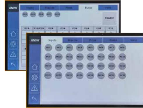
The diagnostics interface is a masterpiece. Service technicians can monitor each inlet and outlet of the control electronics, and can activate each single movement of the machine for setup or error detection.
