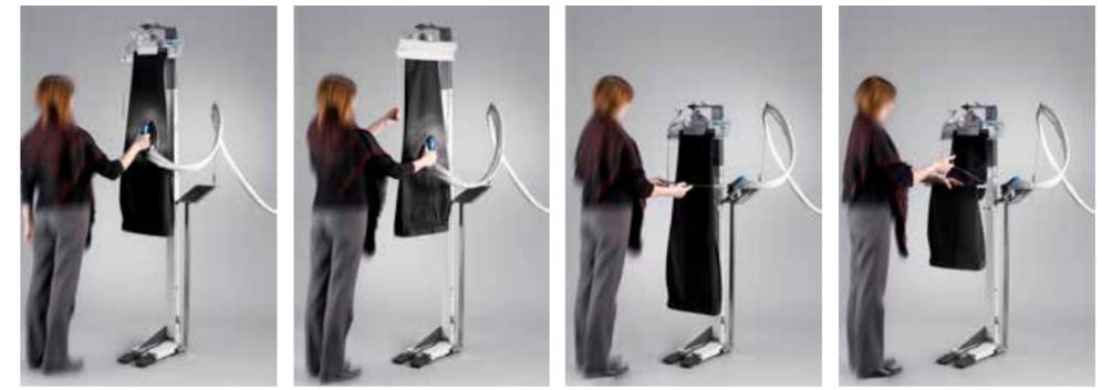
Side stand for touch up and folding. This stand makes operations faster and easier by avoiding transfer to a different touch up station. The L564 includes a handy all-steam iron, and it plugs directly into Pantastar, with no need for new electrical lines or plumbing. After touching up the trousers, the operator transfers them easily to the hanger. The L564 does not require special hangers.
