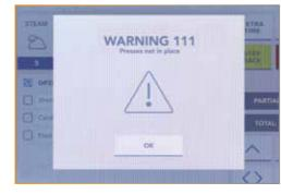
During operation, the error detection program is always active in background. It immediately warns the user in case of anomalies and allows prompt and clear notification to the service technician.
